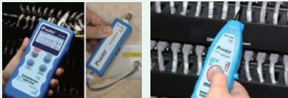
Verify LAN cable condition Wire Hunting and Sorting
